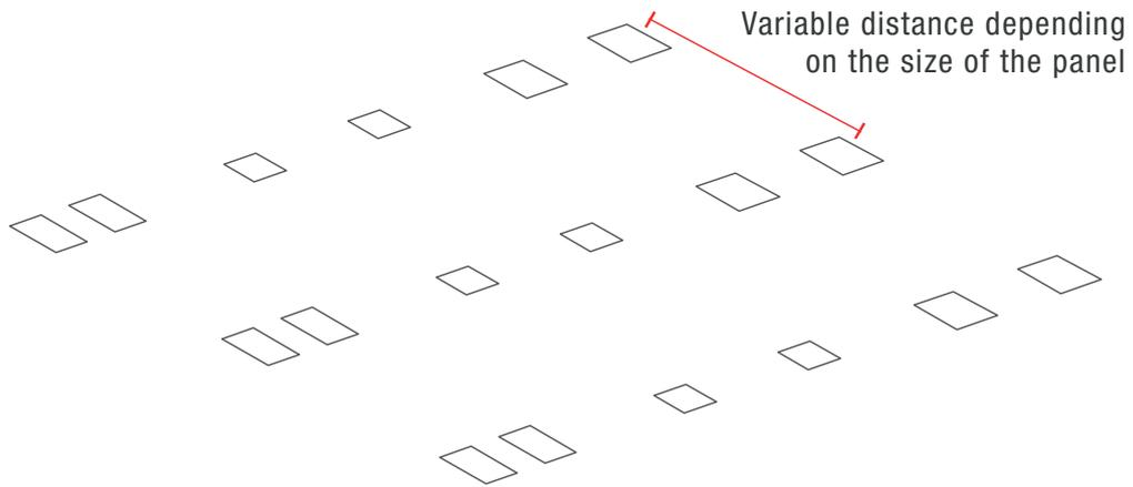
Phase 2: Laying of the ballast on the sheaths
