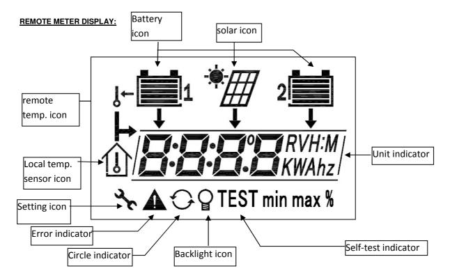
LEDs on the top of the LCD
